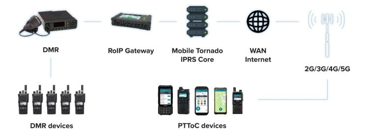
The **RoIP Gateway** can bridge and send audio from a two-way radio network to Mobile Tornado's PTToC application through advanced digital voice processing technology.
